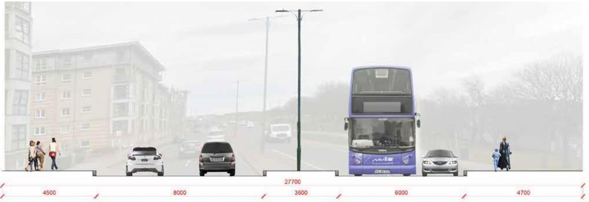
The section above illustrates the current space allocation along Beach Boulevard. The large majority of space is currently allocated to cars and does not contribute to a pleasant pedestrian or cycle environment.
